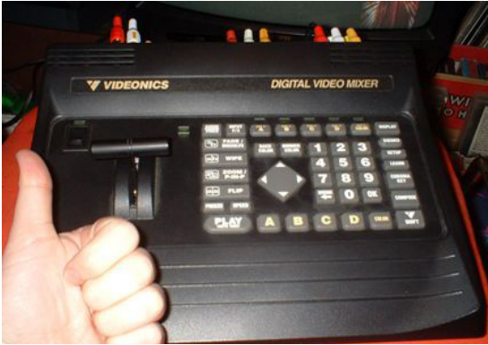
Fig. 3 — The Videonics MX-1 video mixer
