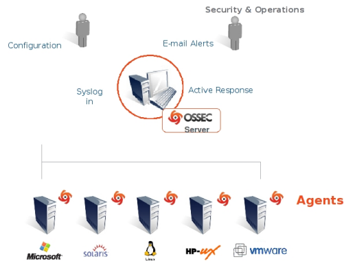
Figure 2.9: Schematic architecture of OSSEC. Taken from: [39]
